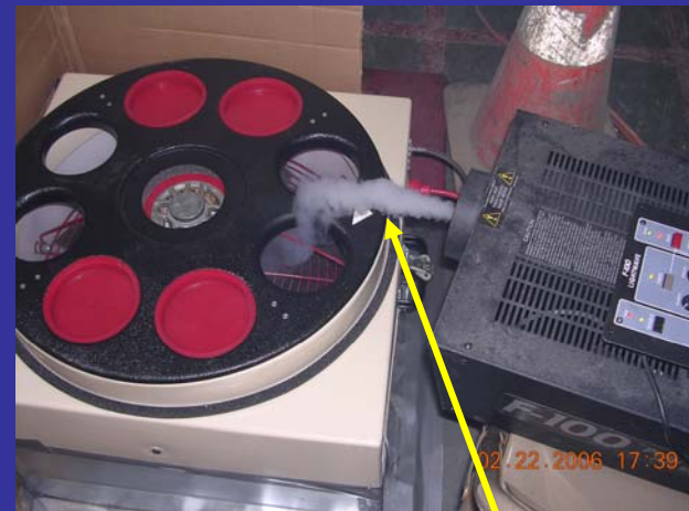
Smoke induced into calibrated fan inlet
